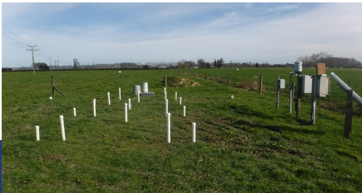
Figure 1: Denitrifying woodchip bioreactor in Hauraki. The high number of sampling wells allows the reaction progress within the bioreactor to be examined.
