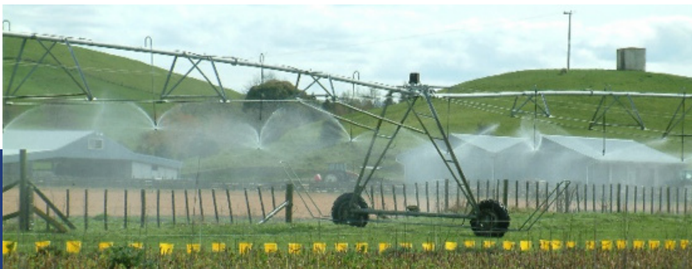
A centre-pivot irrigator about to pass over a row of application depth calibration vessels.
